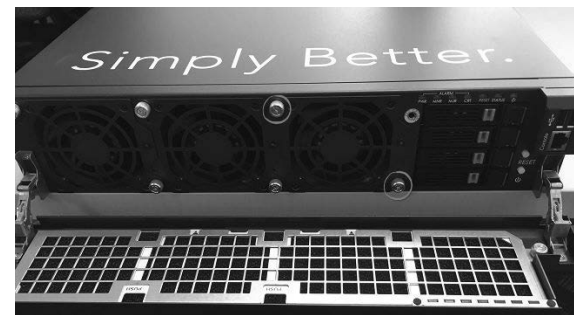
FIGURE 2 Loosen the two thumb screws (circled in red) that secure the fan module
